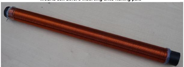
Wound coil adhered onto the fishing pole (note the 10amp strip connector)
